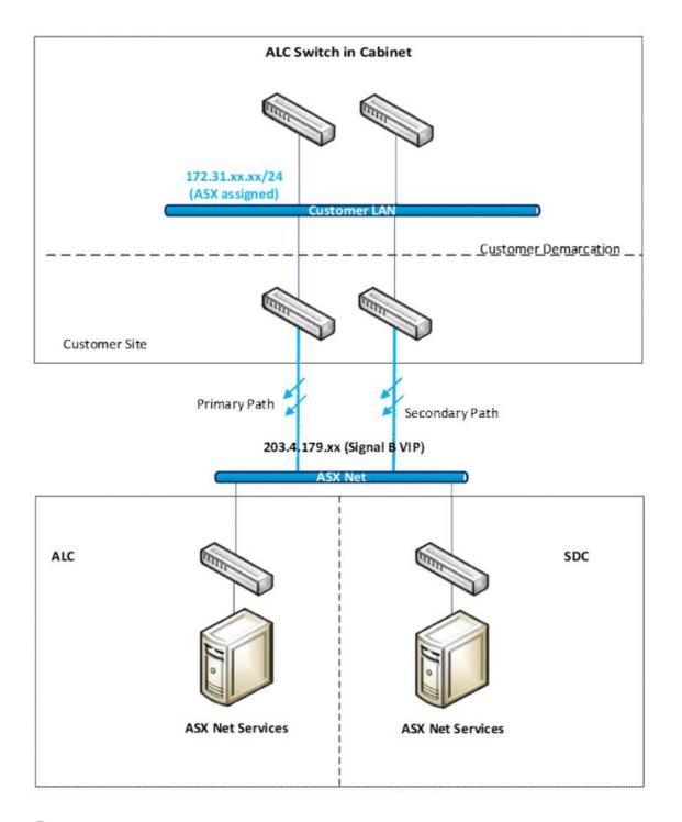
() Note: everything below the customer demarcation line is managed by ASX. As a routine, the ALC-hosted service will be used and in the event of an incident where this service cannot be recovered, ASX will failover customer connectivity to the SDC-hosted service. In both scenarios, the customer will continue to target the same IP and port.
